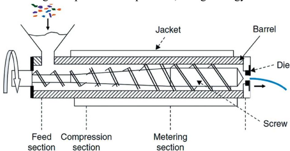
Extrusion also demands good purity. This leads to confusion about what can be recycled. Materials that are a combination of different plastics cannot undergo extrusion. Finally, the strength of extruded plastics dramatically decreases, and they cannot be used in food packaging.
