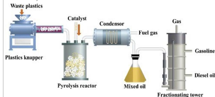
This process can be used in contaminated or mixtures of plastics, including food contamination. The strength is also not compromised, increasing the possible uses. The conversion rate of plastic to petroleum products is 99%. The hot gases generated during the process would be used for heating to make this renewable.
