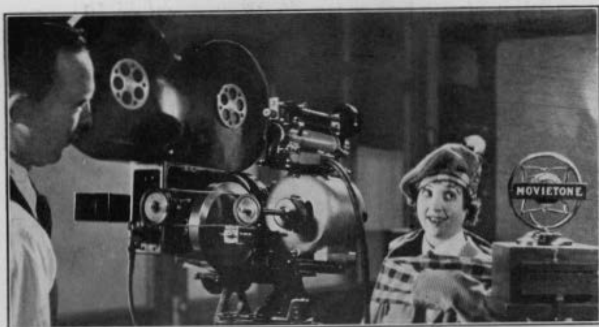
An artist appearing before the microphone and moving picture camera whereby speech and features are recorded simultaneously.
